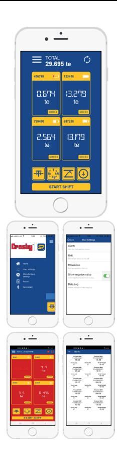
Up to four Crosby Straightpoint, Bluetooth load cells can be connected and monitored by up to eight smartphones, with the HHP2 app installed. It will enable more than one lifting professional to monitor the loads progress and safety, spotting potential dangers or issues from different vantage points.
